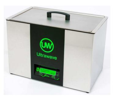
The **Oi-500** is а 33Litre ultrasonic cleaner with a menu driven, LCD control panel. This allows simple adjustment of cycle time (0 to 99mins or continuous mode), temperature (ambient to 80°C), ultrasonic power and frequency mode for precise and accurate processing.
