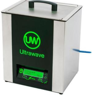
The **Qi-300** is a 17Litre ultrasonic cleaner with a menu driven, LCD control panel. This allows simple adjustment of cycle time (0 to 99mins or infinity mode), temperature (ambient to 80°C), ultrasonic power and frequency mode for precise and accurate processing.
