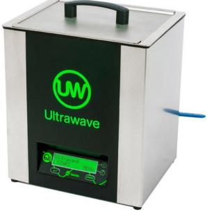
The **Qi-200** is a 12Litre ultrasonic cleaner with a menu driven, LCD control panel. This allows simple adjustment of cycle time (0 to 99mins or infinity mode), temperature (ambient to 80°C), ultrasonic power and frequency mode for precise and accurate processing.
