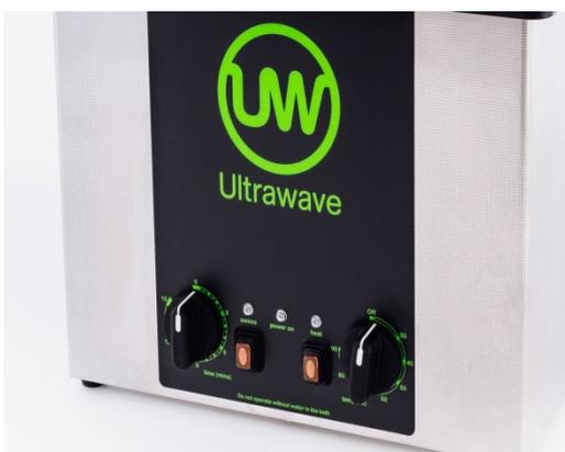
The **U1300H** is a 13Litre ultrasonic bath with heating function reduce processing time.
